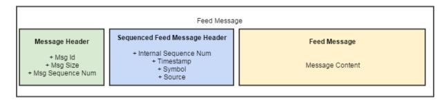
The header contains a total of 31 or 52 bytes, and consists of the following data fields:
