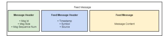
Standard feed message header length is 23 bytes, whereas long feed message header length is 44 bytes. The header consists of the following data fields:
